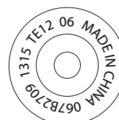
Orifice assembly marking for TE 5 – TE 55
